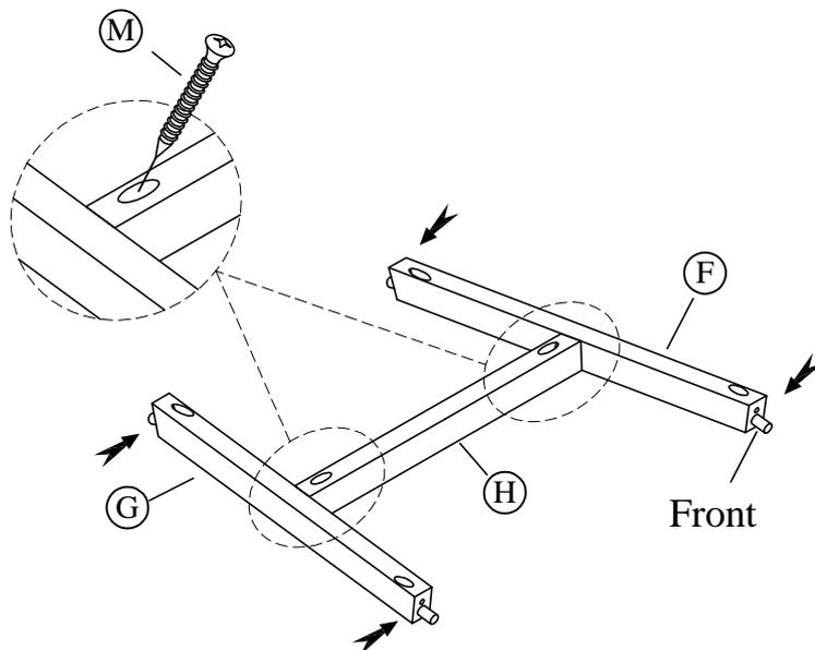
**STEP 4:** Using the Allen key and a Phillips head screw driver, tighten all bolts, then tighten all screws.
